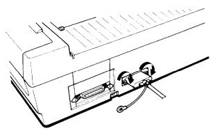
Note: If the screws that come with the cable do not fit into the connector lock nuts on the interface, you need to replace these lock nuts with the optional lock nuts provided with the printer.
